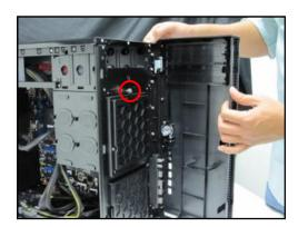
3. Open the drive cage by loosening the top thumbscrew.
